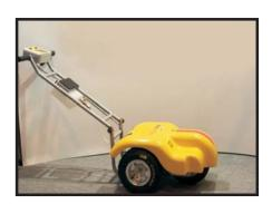
micro GripTester is a cost effective and dynamic alternative to Pendulum spot measurements
